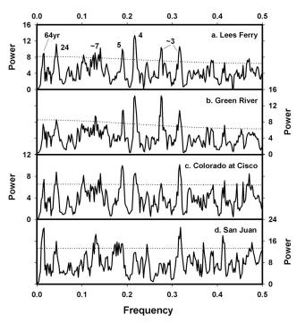
**Figure 6.** Multitaper method spectral analyses [Mann and Lees, 1996] of reconstructed flows for (a) the Colorado at Lees Ferry, Arizona, (b) the Green River at Green River, Utah, (c) the Colorado near Cisco, Utah, and (d) the San Juan near Bluff, Utah. All spectra cover the common period from 1569 to 1997. Peaks are shown versus the 95% confidence level (dotted line). These analyses were performed using a  $3 \times 2$  pi taper under red noise assumptions.
