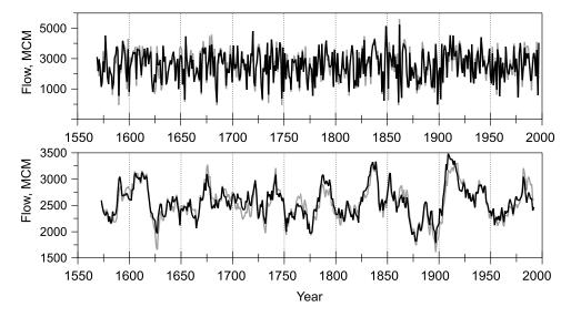
**Figure 3.** San Juan near Bluff, Utah, reconstructed streamflow, 1569–1997, from two models, full predictor pool (gray lines) and watershed-limited predictor pool (black lines): (top) annual values and (bottom) 10-year running average.
