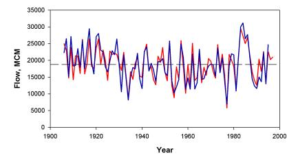
**Figure 2.** Comparison of observed and reconstructed streamflow, Lees Ferry gauge (blue line) and Lees-A reconstruction (red line), 1906–1997 (gauge to 1995).
