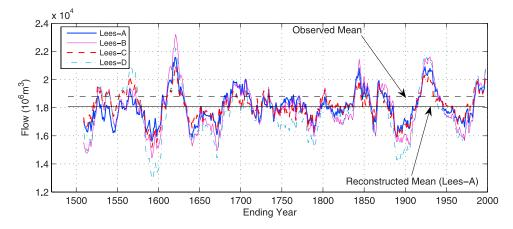
**Figure 4.** Reconstructed 20-year running means of Colorado River at Lees Ferry, Arizona, by alternative statistical models. Horizontal lines are the observed mean of the unsmoothed flows for the 1906–1995 calibration period (dashed line) and the reconstructed mean of unsmoothed flows for the entire (1490–1997) Lees-A reconstruction (solid line). See text and Table 3 for definitions of the models.
