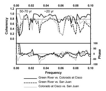
**Figure 7.** Multitaper method cross-spectral analysis [Mann and Lees, 1996] of reconstructed flows at the major subbasin gauges on the Green River at Green River, Utah; Colorado River near Cisco, Utah; and San Juan River near Bluff, Utah. (top) Coherency spectra plotted against the 95% confidence interval (dotted line). (bottom) Phasing of spectral peaks.
